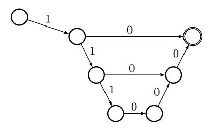
However, this works only for series of 1's and 0's no longer than 3. To handle arbitrarily long strings in this language, the FSM itself would to be arbitrarily big—in which case it would no longer be a *finite* state machine.
