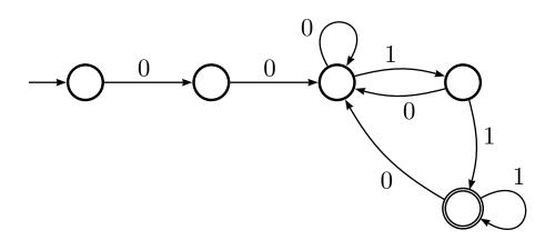
The way to read this is that the left "branch" shows the entry into the system—a string must begin with two 0's. Then transitions happen among the three states on the right, but in order to get to the lower state, we must have come in on a path where the last two inputs were 1's. If we are in that state when the input ends, we accept the string as being in the language. For this reason the final state is also called the *accept state*.
